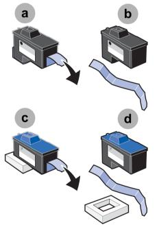
**Warning:** Do not touch the gold contact areas on the back and bottom of the cartridges.
